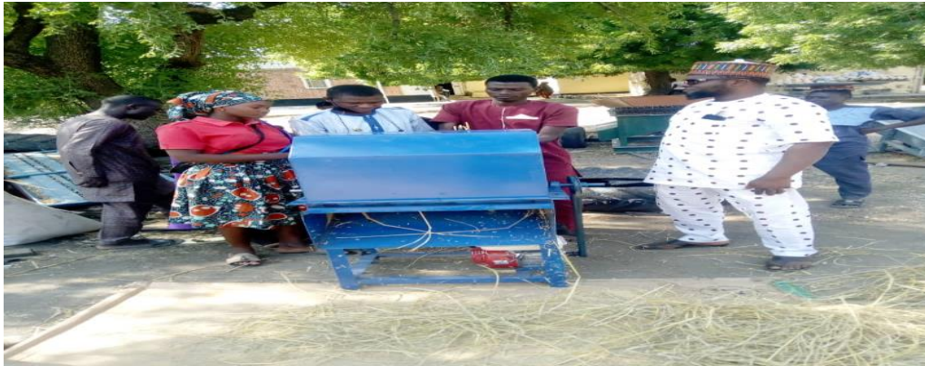
Plate 3.4 Performance test of Mini-rice Thresher
